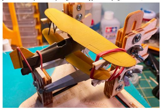
final assembly and some detailing, touch up, weathering and dullcoat.
