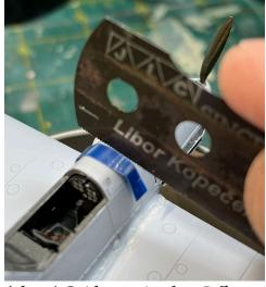
(above) Guide tape in place Jeff carefully makes the first incision. Note that Jeff, (wild man that he is), is dangerously not using the wooden handle with the saw blade. He did this for clarity in this photo.
