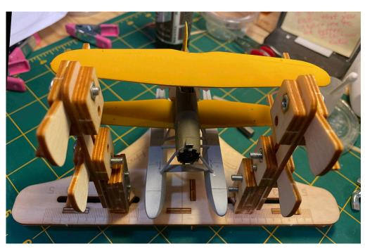
(Above) The nearly completed jig, I just have to glue the rubber cushioning to the upper surfaces so the model rests on rubber and not harder wood.
